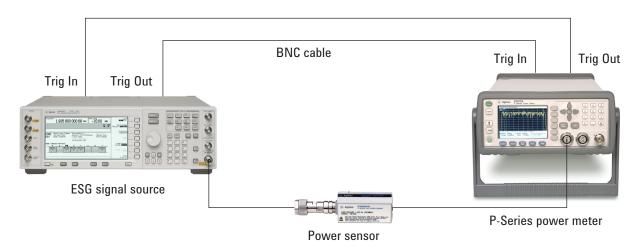
Figure 5. 2-way external triggering setup diagram
