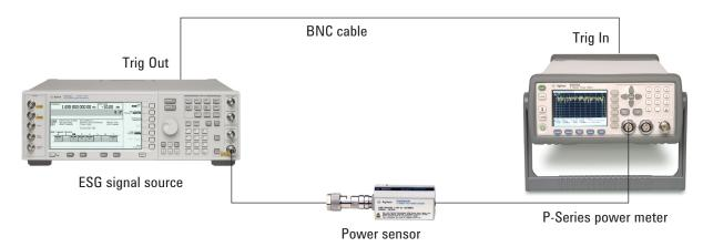
Figure 4. 1-way communication external triggering setup diagram
